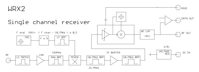
Figure 2: WRX2 block diagram
