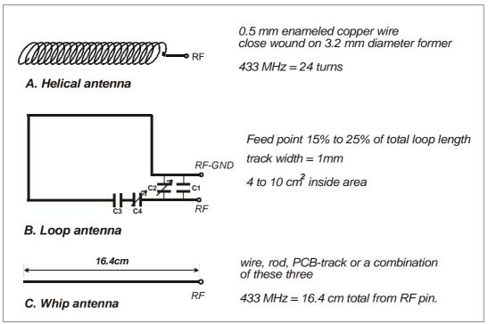
Figure 5: integral antenna configurations
