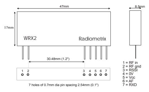
Figure 3: WRX2 pin-out and dimension (with can)
